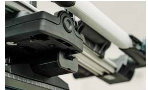
T-bolts inserted in T-Tracks (20 × 20 mm),
